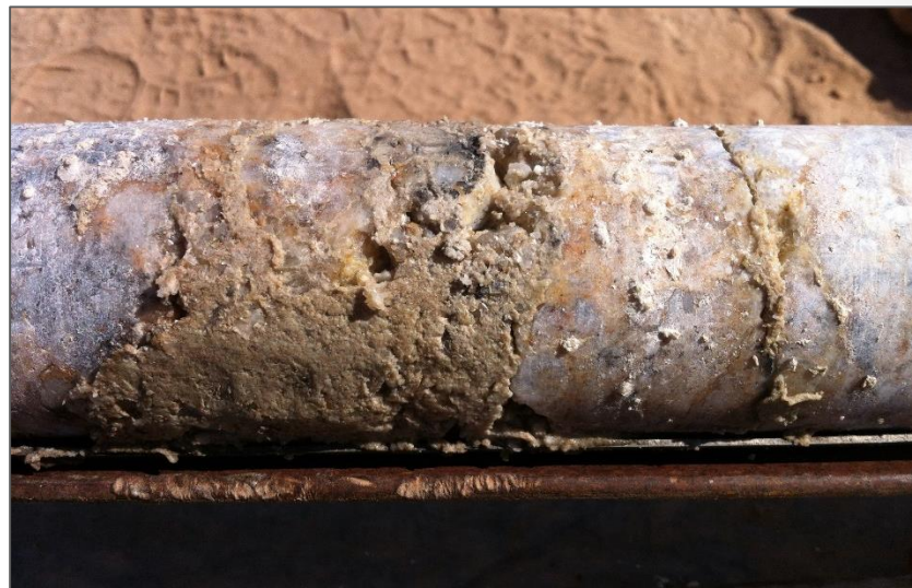
Good recovery in difficult drilling conditions – clay alteration of lithium and feldspar minerals mixed with hard quartz
